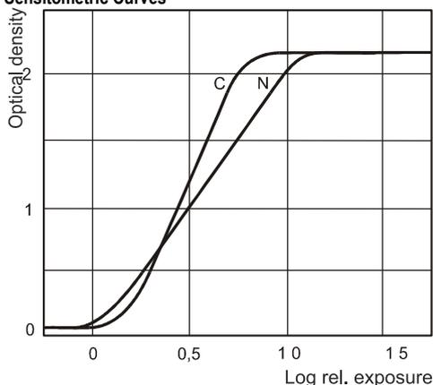
The above shown curves are valid for the glossy surface. Any other surface, namely the matt one, causes a decrease in the maximum density value. According to the ISO standard, the following sensitometric values correspond to the individual contrast grades:
